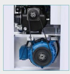
Belt tensioning is effected by means of a motor rocker. The optimum sling arrangement of the belt around the pulley ensures even better power transfer.
