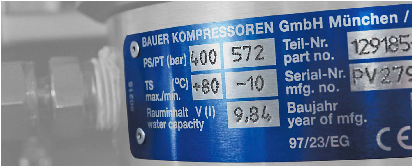
Final separator approved for high temperatures
