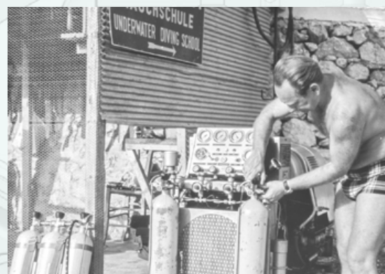
A KA 15-B breathing air compressor in use on a dive base in the late 60s.
