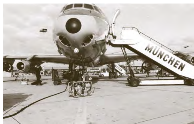
A BAUER high pressure compressor at Munich airport supplies the air to start the turbine.
