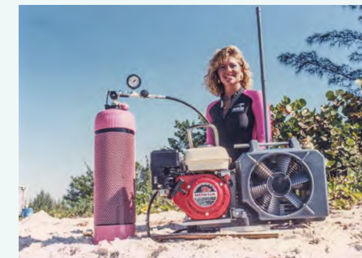
Affordable compressors, such as the UTILUS U10 shown here, enabled each diver to own their own compressor.
