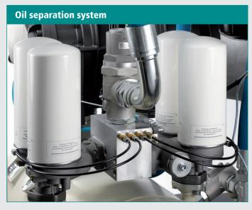
Compressors up to 160 kW are equipped with external separators which can be changed in a simple spin-off/spin-on process. Larger units have an internal separator cartridge. Due to the excellent separation efficiency of the system as a whole, the compressors can be used in the pressure range of 5.0 to 15.0 bar. Special pressures on request.
