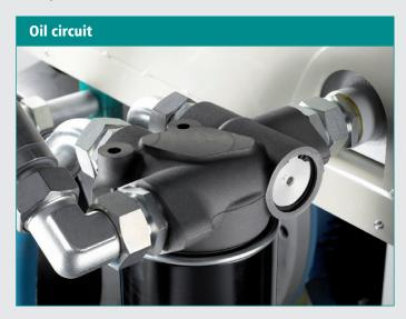
The amount of oil in the units is determined in such a way as to extend the oil change intervals (depending on ambient conditions). An oil level sensor is integrated as standard and is read by the controller. All the units in this series have a horizontal oil separation vessel in which the oil is separated from the compressed air highly efficiently at low speeds. The large surface area of the oil in a horizontal oil separation vessel is a major factor in the prevention of foam build-up.
