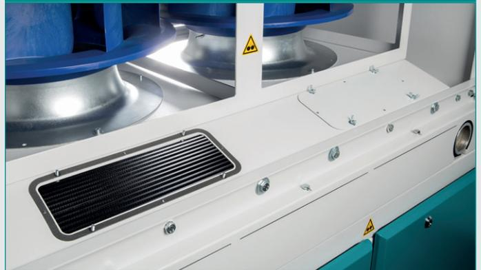
The horizontally mounted cooler can be cleaned by cleaning lids. Alternatively the cooler can be pulled out like a drawer for the purpose of cleaning. Thanks to well dimensioned after coolers for oil and compressed air as well as the integrated oil temperature control, the compressors run reliably even at high ambient temperatures.
