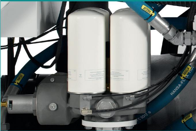
Compressors up to 127 kW are equipped with three or four external separator cartridges which can be changed by a simple spin-off/spin-on procedure. Thanks to the outstanding separation efficiency of the entire system, the compressors can be used in the pressure range from 5,0 to 15,0 bar.
