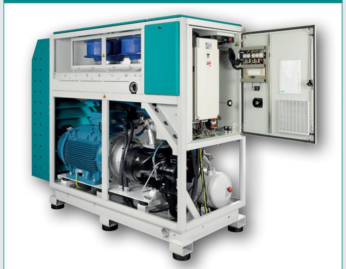
The maintenance parts are easily accessible thanks to removable doors and hinged rear duct silencer. In order to access larger components like motor or air end, the longitudinal bracing can be removed. The separate switch cabinet ensures access to the electrical components.
